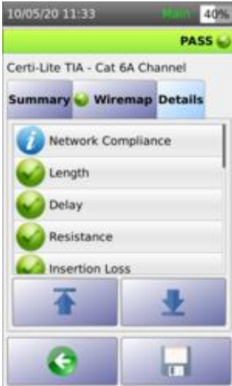
Certi-Lite CAT6A Channel Test
